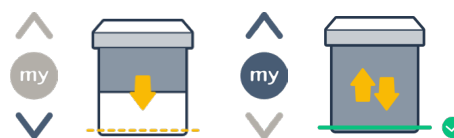
Motor jogs to confirm lower limit
